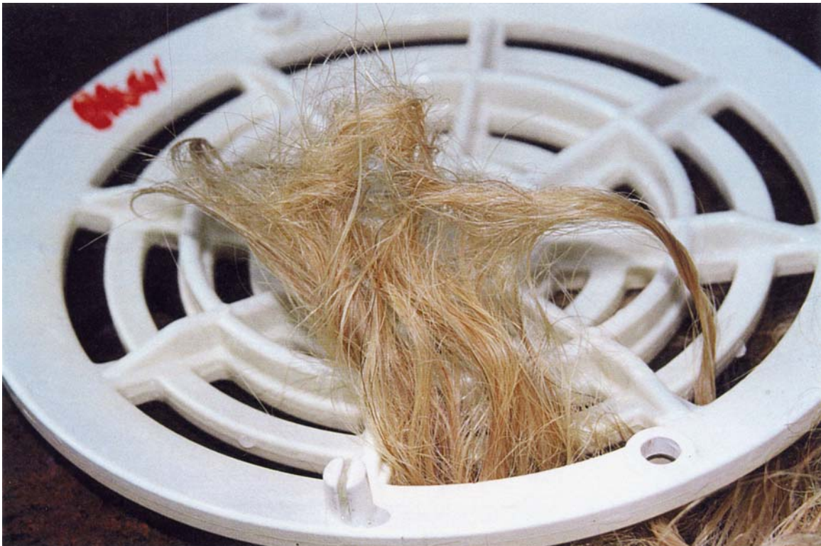
Figure 7 - Underside of a suction cover after attempts to dislodge the tangled natural hair wig by pulling up with the scale and by hand failed. This is not necessarily the suction cover in any other figure(s).
